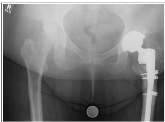
Figure 3: Pre-operative x-rays demonstrating a fracture of the femoral components distal to the modular junction
