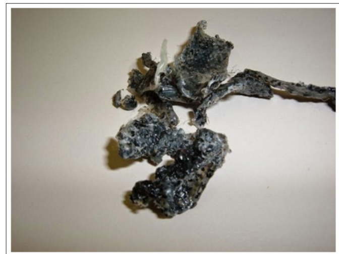
Figure 2: Charr Buildup (Source: https://www.keystoneparts.com/blog/char-buildup-in-glue-melter )
