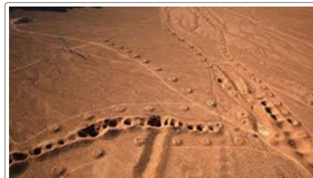
Figure 4: QANAT borehole lines and sinkholes between the lines of boreholes where salt has dissolved
