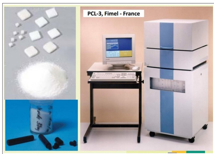
Figure 14: Thermoluminescence dosimetry at the Equal - ESTRO laboratory used for remote dosimetry audit purposes [22]
