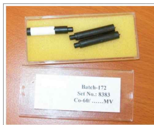
Figure 4: A set of TLDs that contains two dosimeters and one control dosimeter (marked in white) to detect environmental influences and storage of the dosimeters. The dosimeter consists of LiF powder, with the plastic capsules are filled [7]
