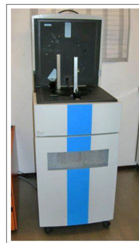
Figure 3: Automatic TLD Analyzer - PCL3 (Fimel, France) used to determine the readings of irradiated thermoluminescent dosimeters-TLDs in the IAEA Dosimetry Laboratory [7]
