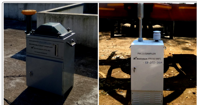
Figure 2: Respirable Dust Samplers (Envirotech APM 460) and PM 2.5 Sampler (Envirotech APM 550 MMFC)
