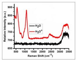
Detection of water (H<sub>2</sub>O) and hydronium (H3O<sup>+</sup>) in water
