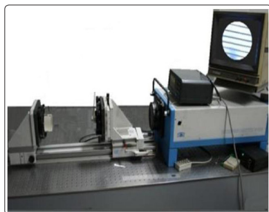
Figure (2-c): Fizeau Interferometer device
