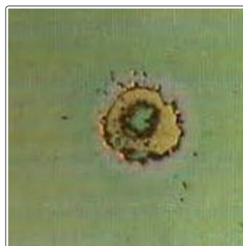
Figure (5-b): Digital image of laser spot on the sensitive burning paper
