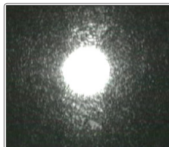
Figure (5-a): Digital image of laser spot on the optical surface
