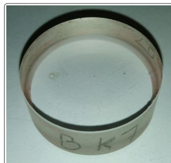
Figure (4-b): The thermal effect of laser presented as spots on the clean glass BK7
