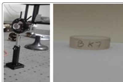
Figure 3: shows the two-sided parallel plate after manufacture, and how to place it on a mechanical stand against lasers
