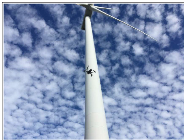
Figure 25: Quadrotor Drone Flying in a Wind Farm Located in Vieira do Minho, Braga (Portugal), for the Inspection of the Nacelle and the Blades in One of the Wind Turbines (author's Photograph)
