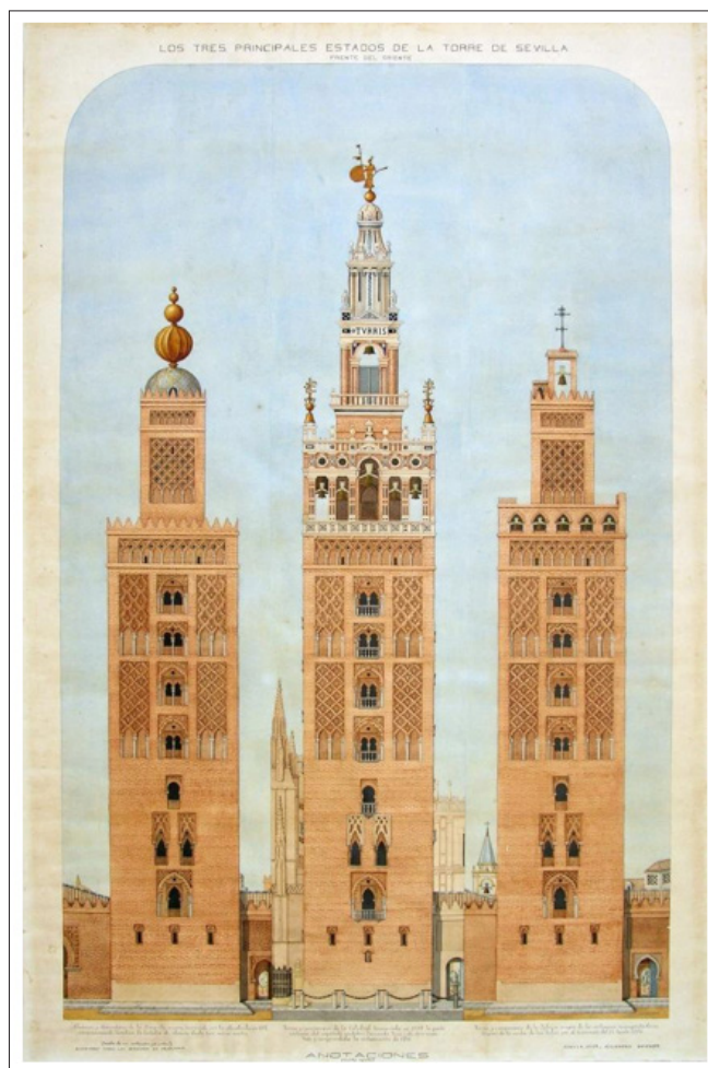
Figure 5: Drawing by Alejandro Guichot (1909) representing the Giralda Bell Tower, in Three Different Elevations: Its Three Phases of Construction. It is a Watercolor Outlined With a Nib [11].
