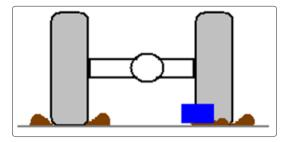
Shown here is the rear axle of the car — a rear view and a scraper behind the right wheel. One scraper on the right wheel is enough. The scraper shifts only one snow roller into its own track. Of course, it is better on both wheels, but this is enough to prevent ruts in deep snow.
