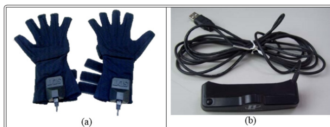
Figure 3: (a) 5DT Data glove 5 Ultra (b) InterTrax2
