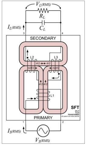
Figure 4: Schematic of SFT Output Section
