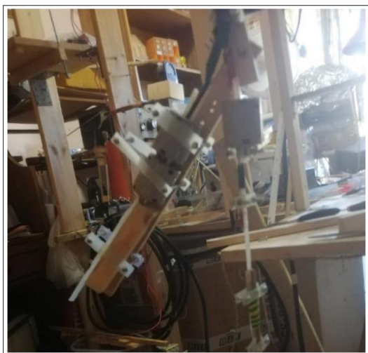
Pendulum: V-shaped FLEXIBLE dipole arm about 14.5 cm long SETUP: 2 cylindrical ferrites clamped on fixed arm (mass - braid)
