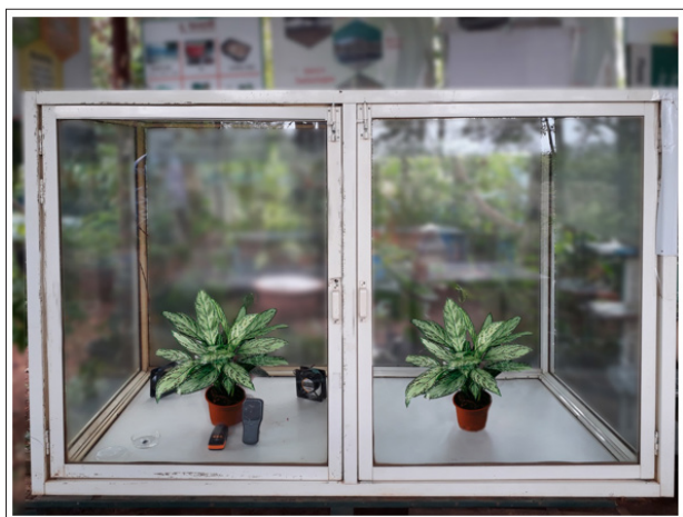
Figure 1: Exposure chamber with Aglaonema commutatum (representative plant)
