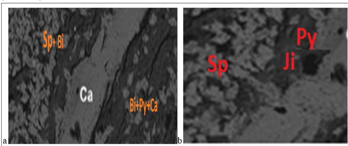
**Plate III:** Reflected light microscope of manganese nodules from Madaka quarry area(a) spalerite-birnessite in a rhombic crystals (Sp + Bi) surrounded by pyrolusite (Py) and crosscut by a post-accretional crack filled with calcite (Ca) and (b) Spalerite (Sp) grains scattered within the nodule.
