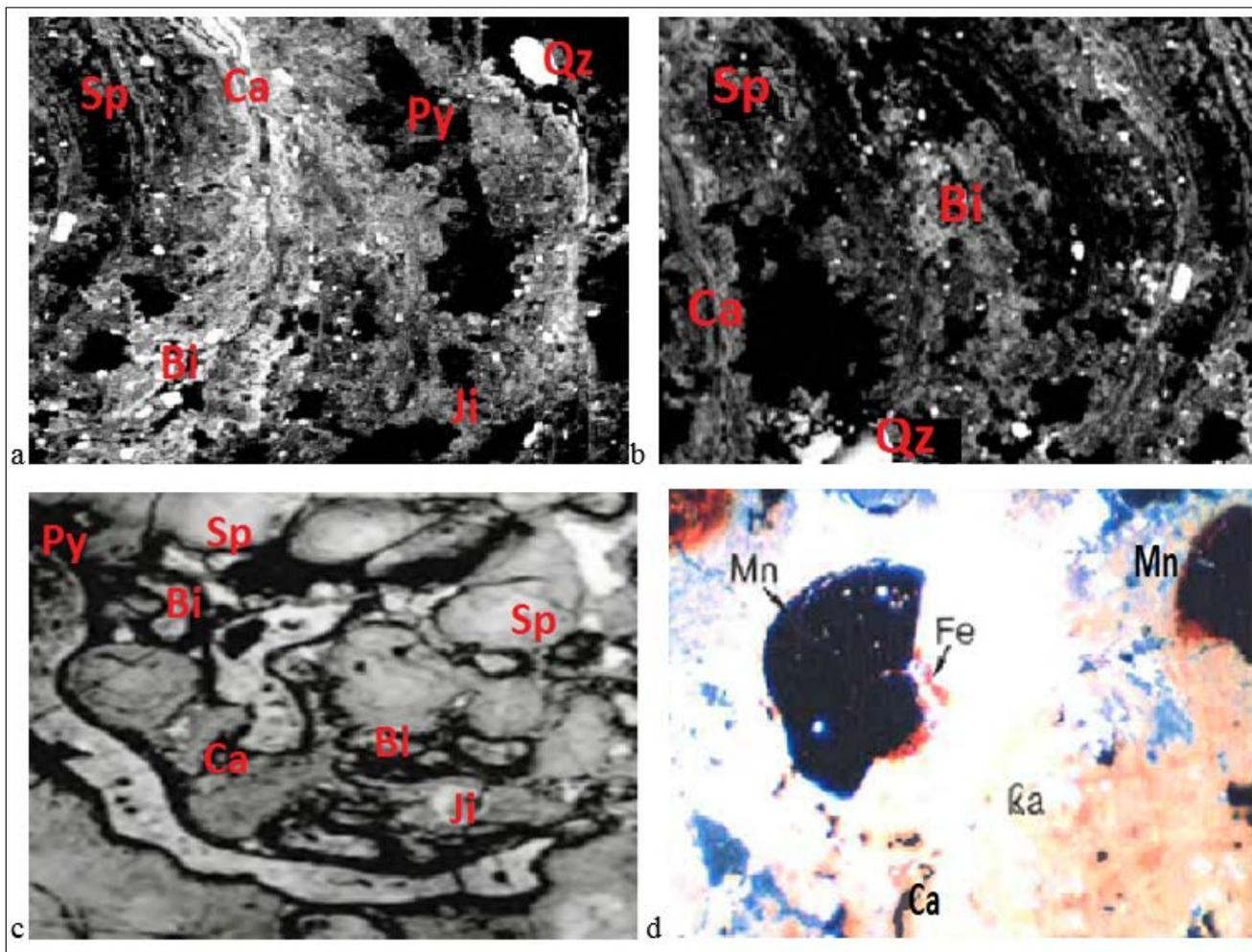
**Plate II:** Reflected light microscope of nodules from Madaka (a) a crystal of spalerite-birnessite surrounded by pyrolusite (Py), (b) Spalerite (Sp) filling a post-depositional crack in disperse or forming aggregates (C) partially pseudomorphed by spalerite which is paragenetic with Fe-Mn rhombic crystals (Sp + Bi) and (d) Rhombic crystal of iron and manganese within the nodule with the calcite filling the void space.
