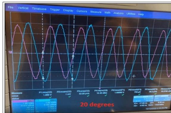
**Figure 5:** Oscilloscope Trace of Amplified Signals at 20° Rotation into Phase-Frequency Detector Circuit. Horizontal Scale has 5 ns/div; the Vertical Scale is 1 V/div
