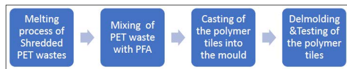
Figure 3: Production process of the tile
