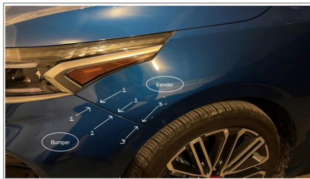
Figure 1: Gap Present between Bumper and Fender on Left-Hand Side
