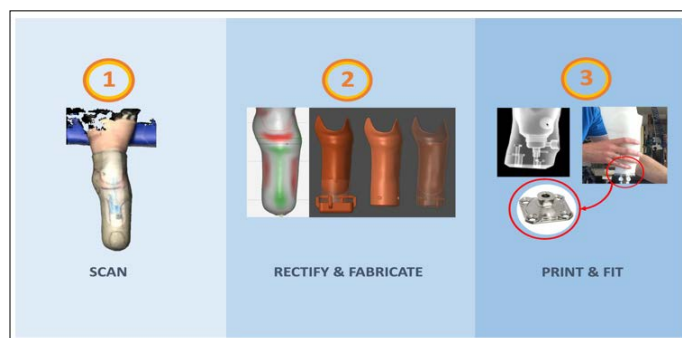
Figure 1: Visual Representation of 3D Scanning (1), Rectification & Fabrication (2), and Print & Fit (3) Steps Involved in the Production of 3D Printed Transtibial Sockets
