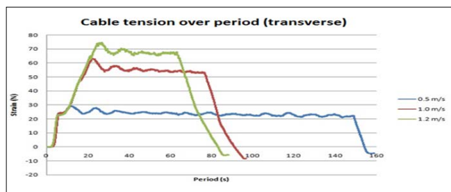
Figure 9: Cable Tension at Different Current Velocity (90 degree)
