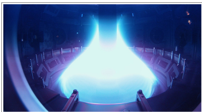
Figure 3: Hot Plasma, Magnetically Confined in a Tokamak
