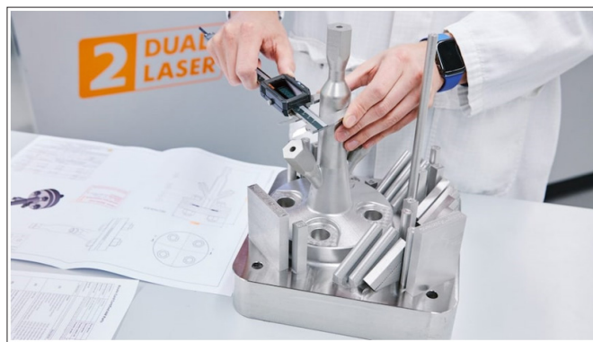
Figure 2: 3D Printed Pressure Vessel that Obtained CE Mark [7]
