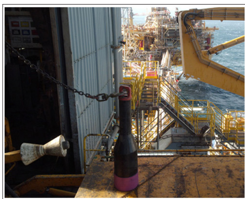
Figure 1: Waterbushing Manufactured with WAAM (Courtesy of Total Energies / Vallourec) [6]
