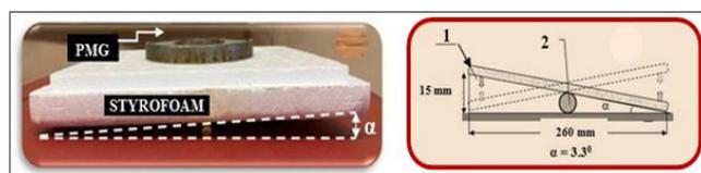
**Figure 7:** Experimental setup: (a) general view, (b) schematic diagram for creating EVL with an oscillation frequency in the range of 2–5 Hz (1 is the Styrofoam as a fit bed for the PMG, 2 is the cylinder of 7-mm diameter).
