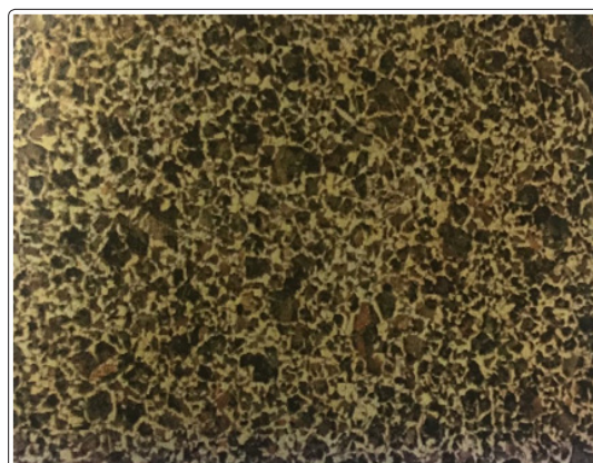
Figure 5: Micrograph of Exposed Reinforcement Bar. The Microstructure Consists of Uniform Distribution of pearlite (dark patches) and Ferrite (white patches). (x200)
