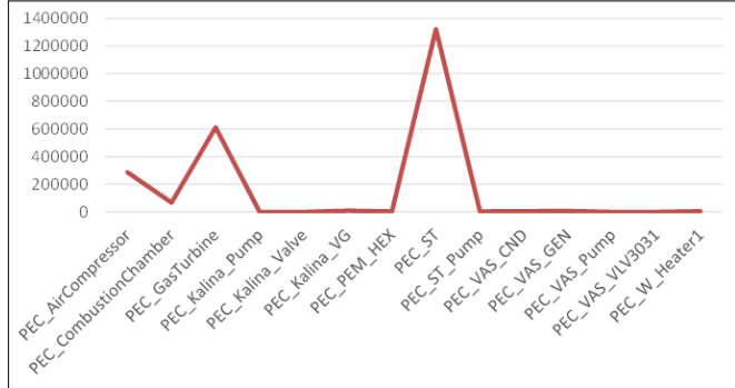
Figure 25: purchase equipment cost, PEC for each component of the proposed power plant
