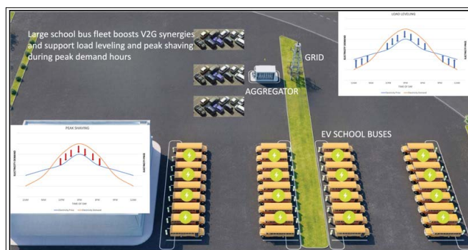
Figure 5: Big EV School Bus Fleet to support the V2G Grid during Peak Demand Hours
