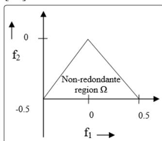
**Figure 2:** The non-redundant region for the calculation of bi-spectral frequencies
