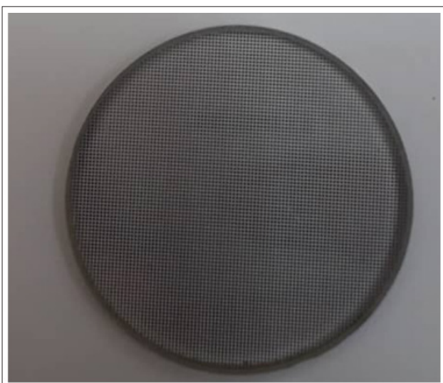
Figure (3-C): A digital image of the half-reflective plate of light after chess paint, Fresnel reflection coating and vertical positioning method.
