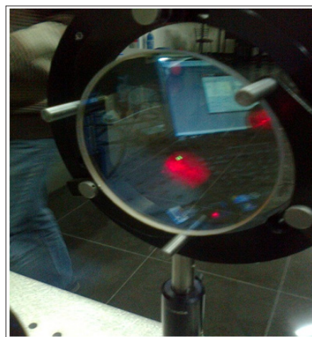
Figure 5: Real image of the semi reflective plate during testing.
