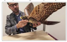
"Robird", developed by Dutch firm Clear Flight Solutions, looks and flies like a real bird, but requires an operator for take-off and landing. Photo: YouTube
