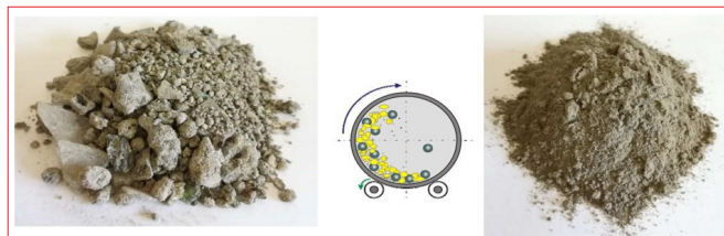
Figure 3: Working process of a ball mill usually used in the first stages of a laboratory analysis, as a pretreatment process of physical nature, consisting of the fragmentation of slags for the purpose of reducing the particle diameter [107].
